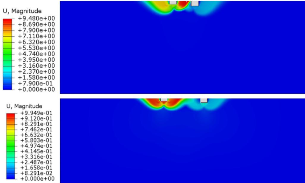
Figure 12. Total displacement contour for  $D_L/B = 0.5$  and  $D_R/B = 0.75$
