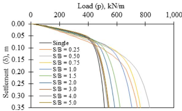
Figure 3.  $p-\delta$  behaviour for  $D_L/B = 0.5$  and  $D_R/B = 0.5$
