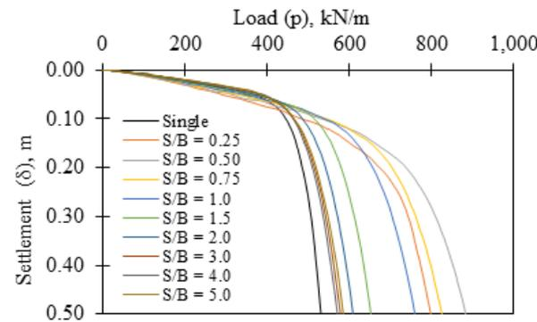
Figure 4.  $p-\delta$  behaviour for  $D_L/B = 0.5$  and  $D_R/B = 0.75$
