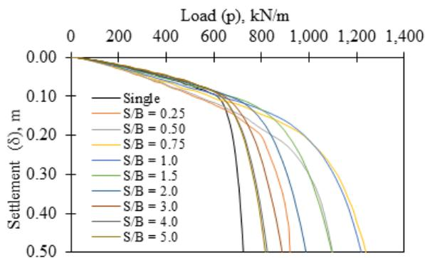
Figure 8. p- $\delta$  behaviour for  $D_L/B = 1.0$  and  $D_R/B = 1.0$
