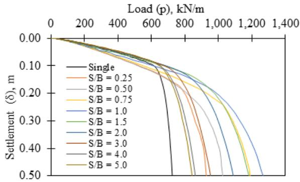
Figure 6. p- $\delta$  behaviour for  $D_L/B = 1.0$  and  $D_R/B = 0.5$
