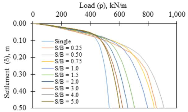
Figure 7. p- $\delta$  behaviour for  $D_L/B = 1.0$  and  $D_R/B = 0.75$
