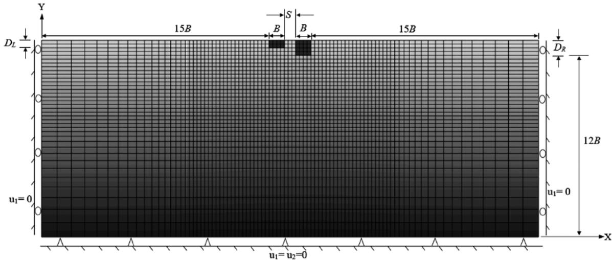
Figure 2. Discretisation of domain and boundary condition
