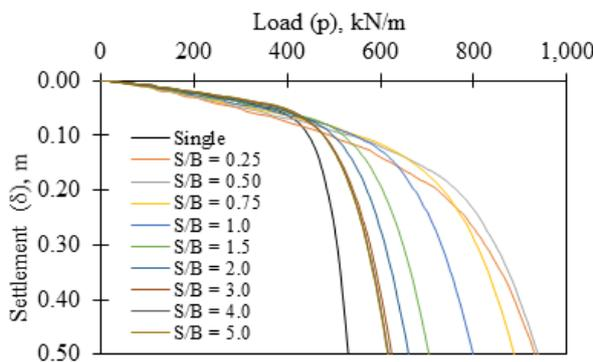
Figure 5.  $p-\delta$  behaviour for  $D_L/B = 0.5$  and  $D_R/B = 1.0$
