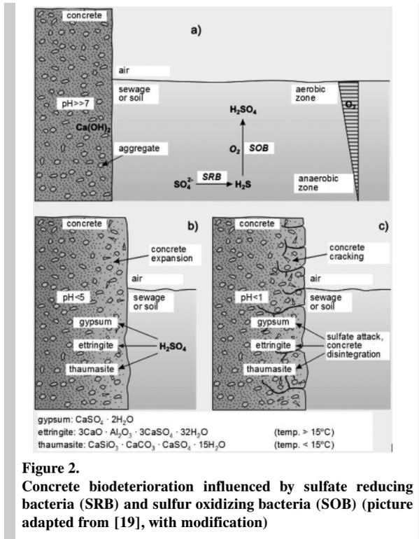
**Figure 2.** Concrete biodeterioration influenced by sulfate reducing bacteria (SRB) and sulfur oxidizing bacteria (SOB) (picture adapted from [19], with modification)
