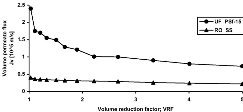
Figure 7. Dependence of permeate flux on volume reduction factor during ultrafiltration and reverse osmosis of landfill leachate purified by means of biological method ( $\Delta P_{(UF)} = 0.2 \text{ MPa}$ ,  $u_{(UF)} = 2.5 \text{ m/s}$ ,  $\Delta P_{(RO)} = 2.07 \text{ MPa}$ ,  $u_{(RO)} = 1.5 \text{ m/s}$ ,  $T = 298 \text{ K}$ )
