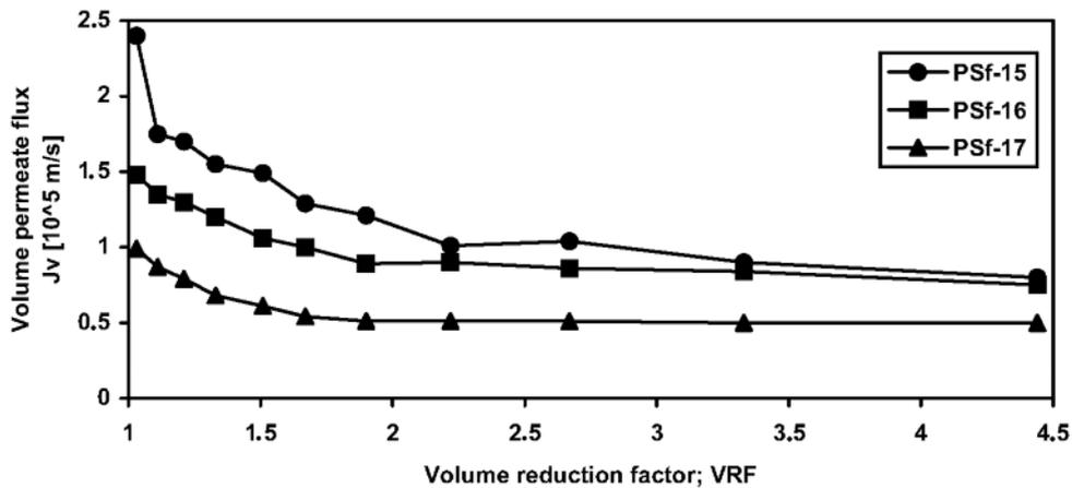
Figure 5. Dependence of volume permeate flux on volume reduction factor for tubular PSf membranes ( $\Delta P = 0.3$  MPa,  $u = 2.5$  m/s,  $T = 298$  K)
