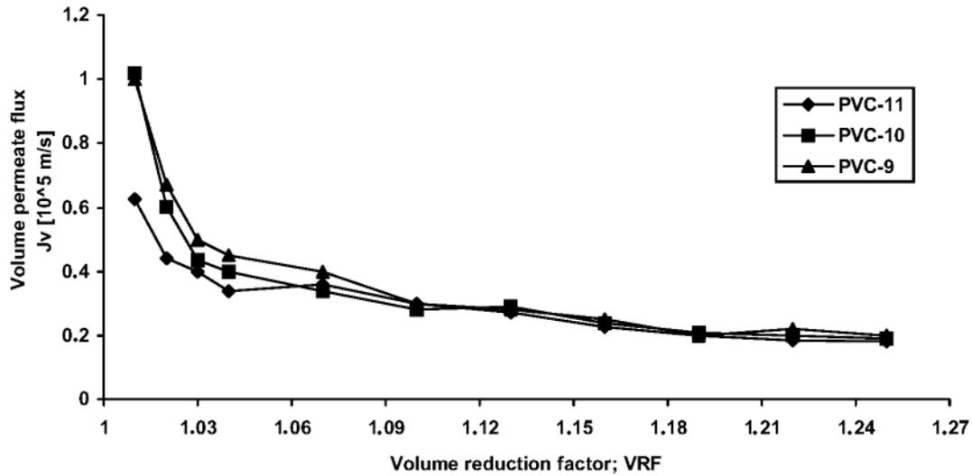
Figure 4. Dependence of volume permeate flux on volume reduction factor for flat PVC membranes ( $\Delta P = 0.3$  MPa,  $u = 1.5$  m/s,  $T = 298$  K)
