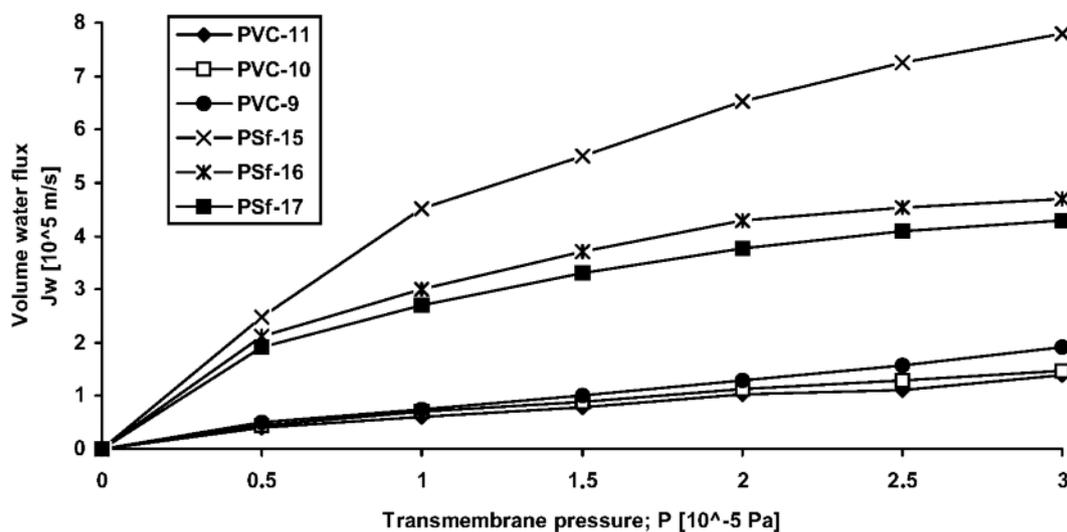
**Figure 2.** Dependence of volume water flux on transmembrane pressure for PVC and PSf membranes of different polymer concentrations in the casting solution
