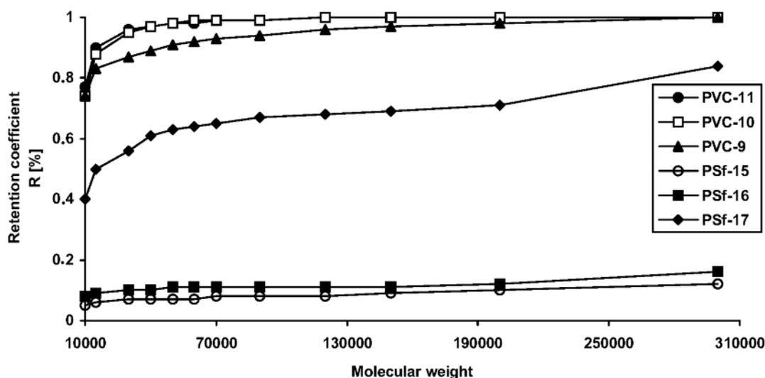
Figure 3. "Cut-off" curves obtained from gel permeation analysis of feeds and permeates for PVC and PSf membranes
