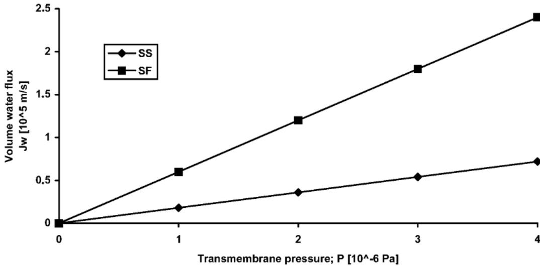
Figure 6. Dependence of water flux on transmembrane pressure for nanofiltration SF membrane and osmotic SS membrane, ( $u = 1.5 \text{ m/s}$ ,  $T = 298 \text{ K}$ )
