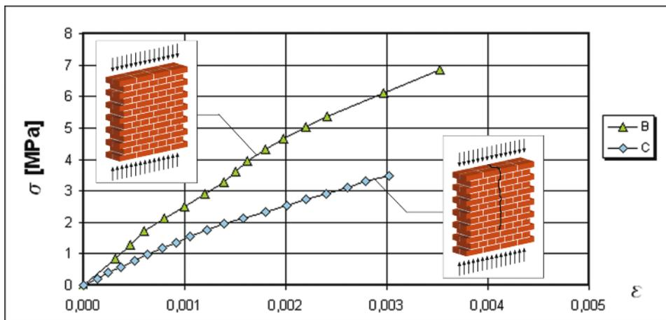
Figure 11. The  $\sigma$ - $\epsilon$  relationships for the B and C series
