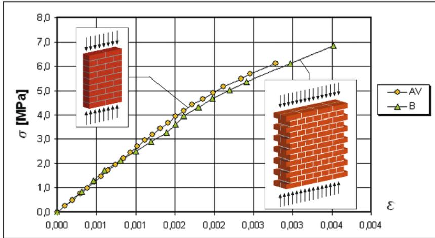
Figure 10. Comparison of  $\sigma$ - $\epsilon$  relationships for un-strengthened and un-cracked samples
