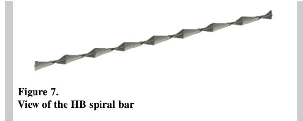
construction including vaults, arches and brick-bridges [14, 15]. Strengthening cracked elements of **E**, **F** and **G** series was carried out by crack stitching with special HB spiral bars (see Fig. 7) of about 6 mm diameter. The bars were made of austenitic stainless steel and embedded in cementitious, thixotropic, injectable, non-shrink HB MM2 grout. Strengthening of the **E** samples (3 specimens – see Table 1) was
