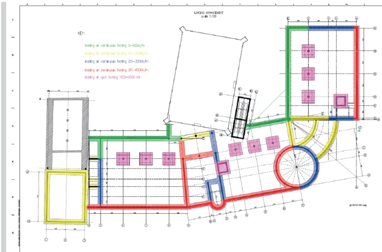
Figure 5. Design loads arrangement
