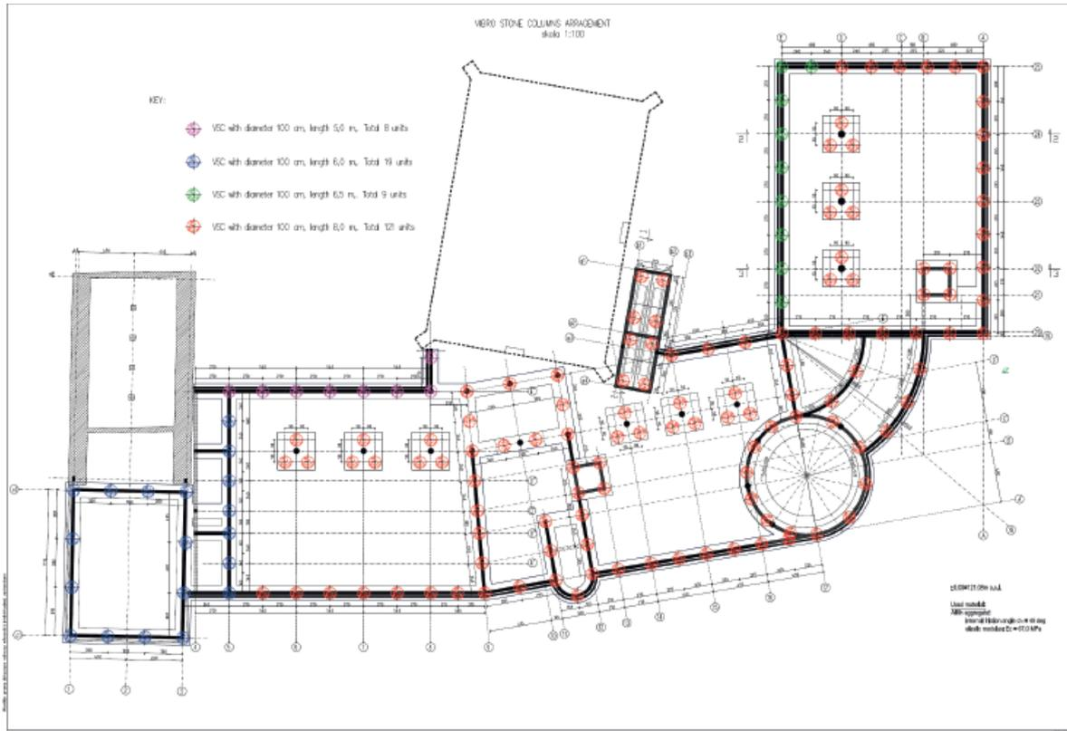
Figure 6. Vibro Stone Columns arrangement [1]
