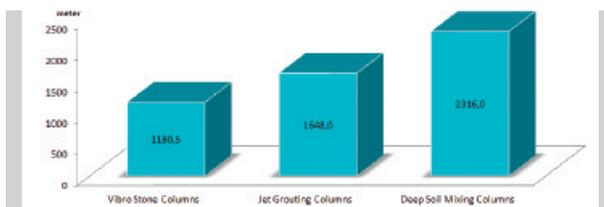
Figure 14. Total costs of forming various types of columns [PLN] [1]
