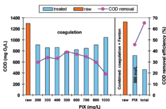
Figure 6. The effectiveness of COD removal by coagulation (pH 5, reaction time = 30 min.) and combined coagulation–Fenton oxidation system (PIX dose = 500 mg/L,  $\text{H}_2\text{O}_2$  conc. = 1350 mg/L,  $\text{Fe}^{2+}/\text{H}_2\text{O}_2$  ratio = 0.2, pH 3, reaction time = 45 min.)
