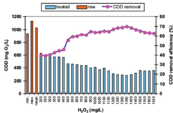
Figure 2. Effect of the  $\text{H}_2\text{O}_2$  dosage on the COD removal efficiency ( $\text{Fe}^{2+}/\text{H}_2\text{O}_2$  ratio = 0.3, pH 3, reaction time 90 min.)
