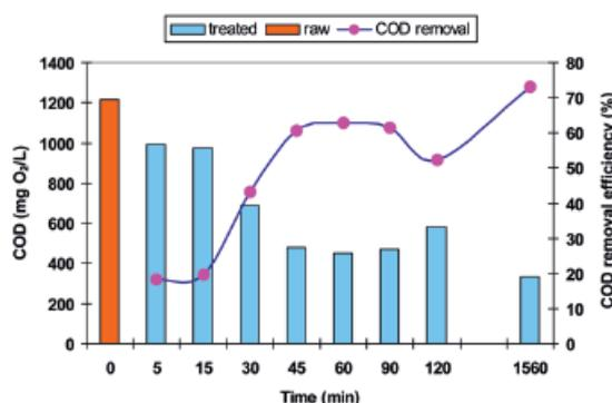
Figure 5. Effect of the reaction time on the COD removal efficiency ( $H_2O_2$  conc. = 1350 mg/L,  $Fe^{2+}/H_2O_2$  ratio = 0.2, pH 3)
