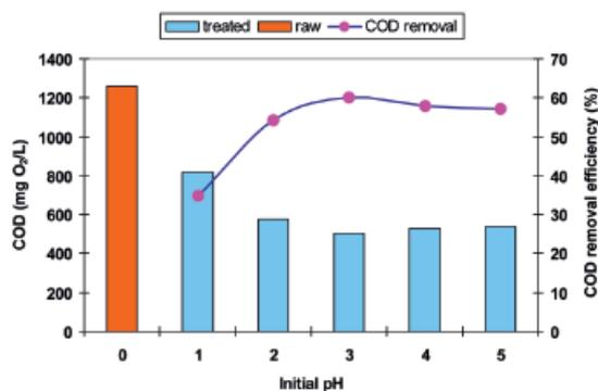
Figure 4. Effect of the initial pH reaction on the COD removal efficiency ( $H_2O_2$  conc. = 1350 mg/L,  $Fe^{2+}/H_2O_2$  ratio = 0.2, reaction time = 120 min.)
