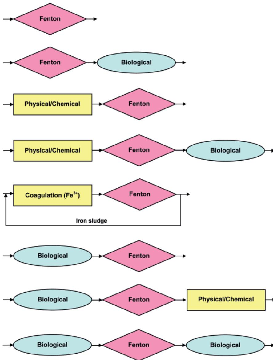
Figure 1. Flow sheets for Fenton treatment of landfill leachate [29]
