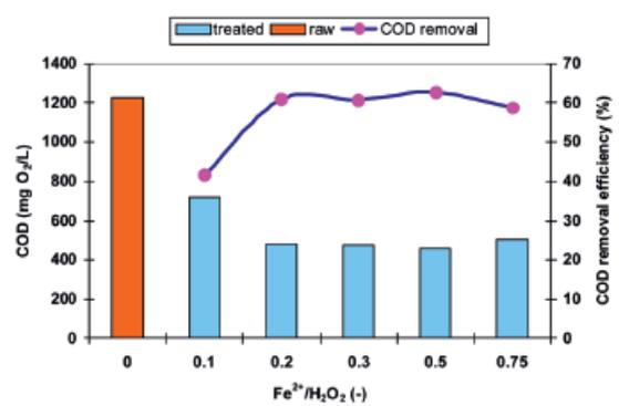
Figure 3. Effect of the  $\text{Fe}^{2+}/\text{H}_2\text{O}_2$  dosage on the COD removal efficiency ( $\text{H}_2\text{O}_2$  conc. 1350 mg/L, pH 3, reaction time 120 min.)
