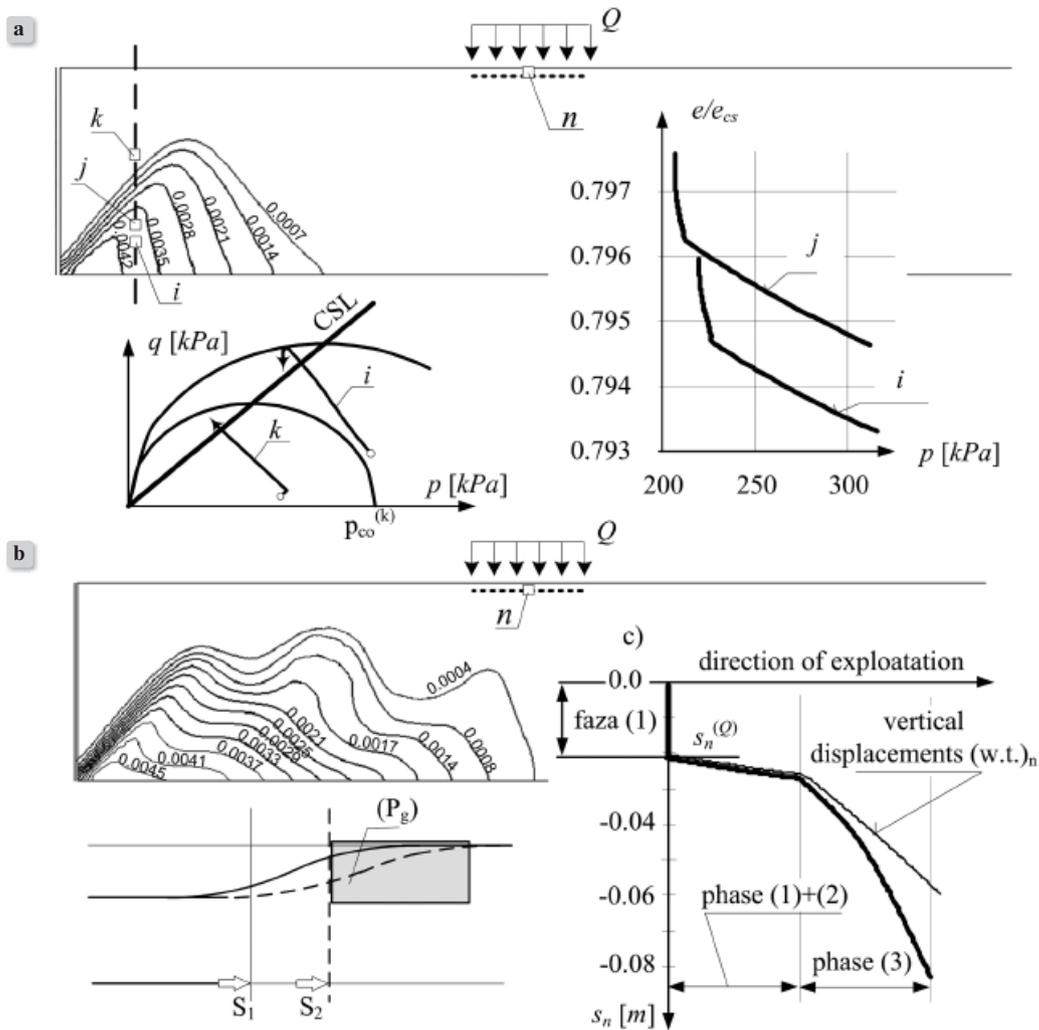
**Figure 6.** Analysis of the areas of subsoil state change in mining subsoil subject to deformations: a) at stopped front of exploitation in point S1, b) at displacement of exploitation front within the range S1–S2, c) impact of another commencement of exploitation on the construction additional settlements
