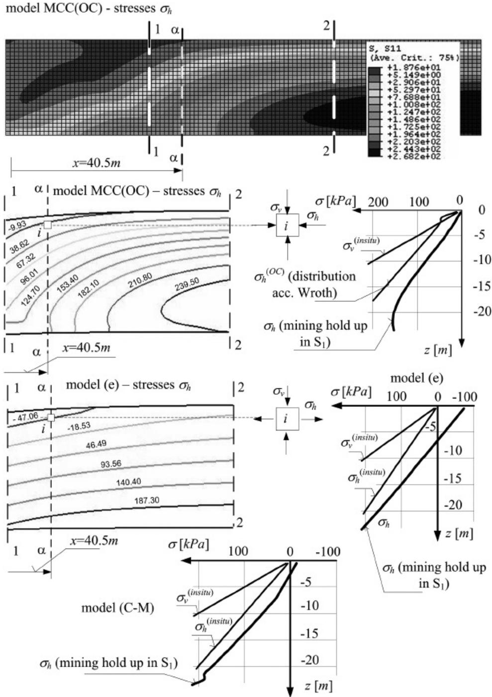
Figure 5. State of stress analysis in mining subsoil subject to deformation a) by means of the described model (MCC), b) by means of models (C-M) and (e)
