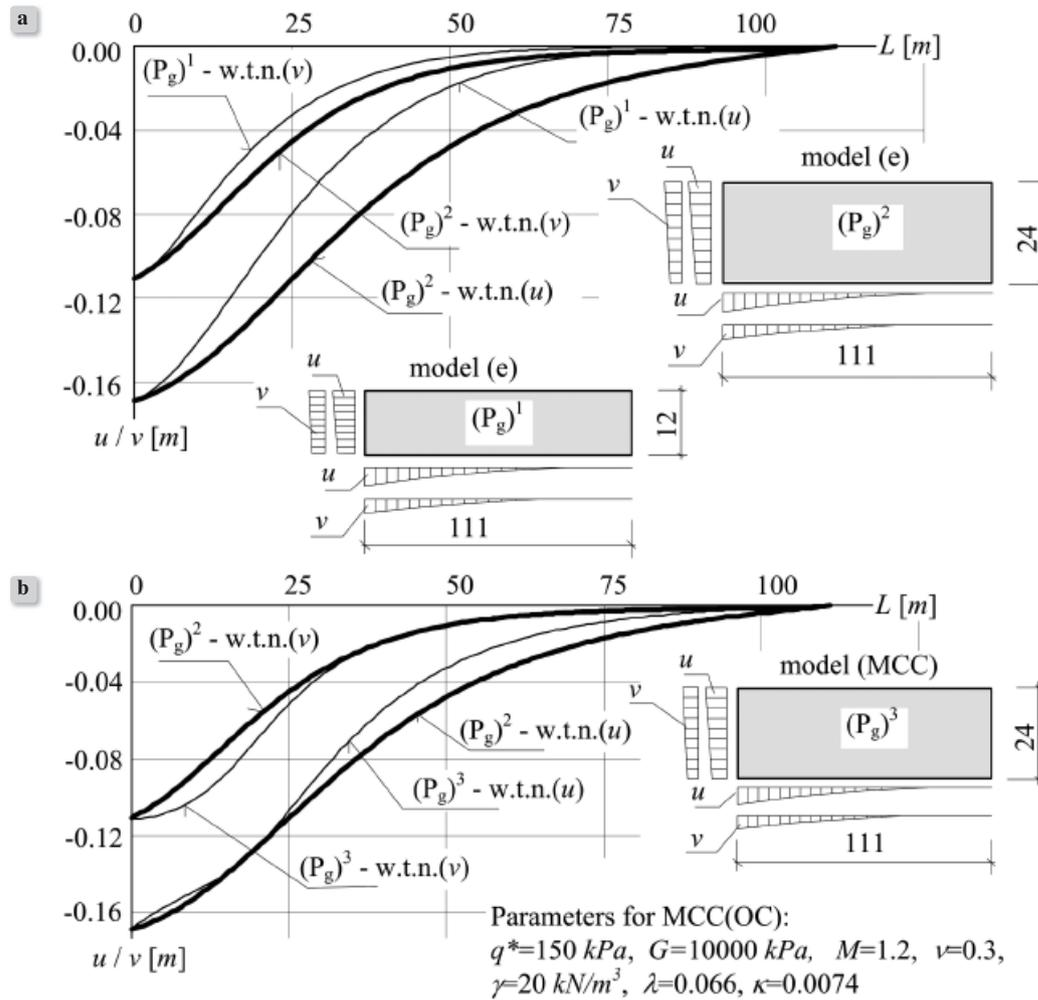
Figure 4. Functions of free area deformations: a) for various heights of the mining subsoil, b) for various soil constitutive models
