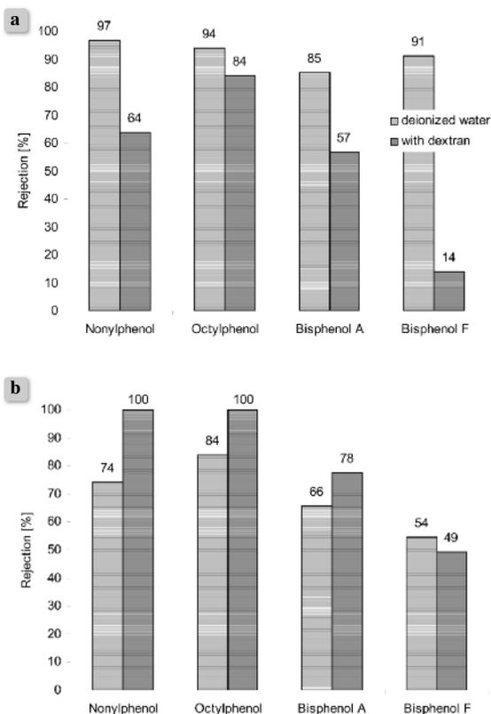
**Figure 4.** Influence of dextran (1000 mg/dm<sup>3</sup>) on xenoestrogens rejection by reverse osmosis (A) and nanofiltration membrane (B)
