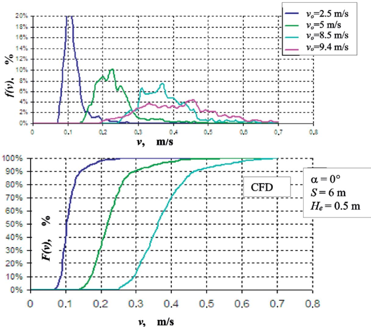
Figure 8. Comparison of the profiles of frequency function and cumulative distribution of the speed in the occupied zone for  $y=1.5$  m for various values of supply air velocity
