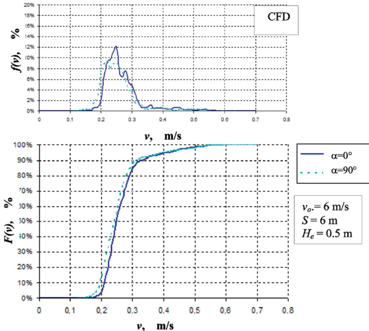
Figure 10. Comparison of the profiles of frequency function and cumulative distribution of the speed in the occupied zone for  $y=1.5$  for various angles of vanes in the inlets
