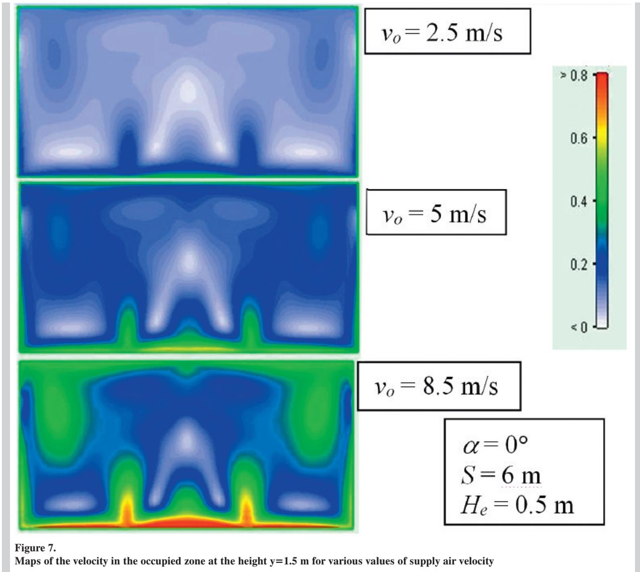
Figure 7. Maps of the velocity in the occupied zone at the height  $y=1.5\text{ m}$  for various values of supply air velocity
