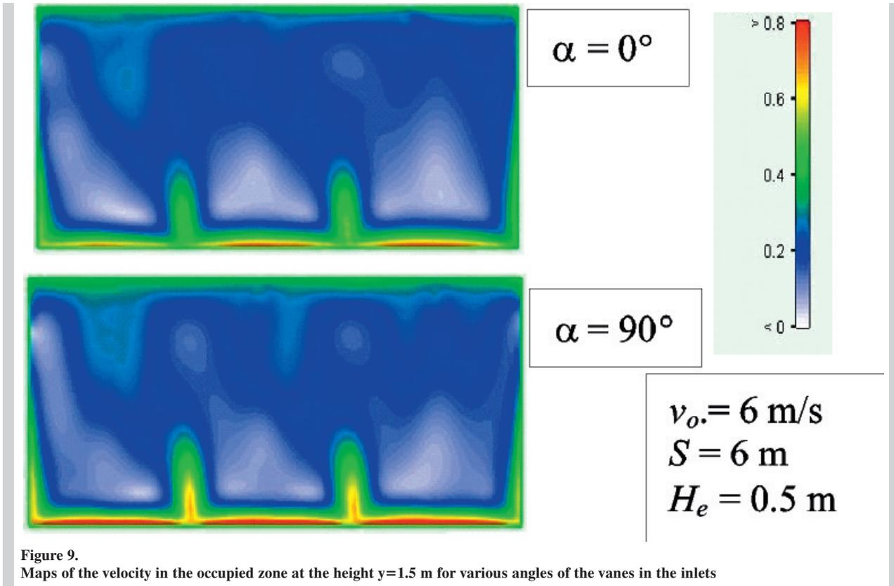
Figure 9. Maps of the velocity in the occupied zone at the height  $y=1.5 \text{ m}$  for various angles of the vanes in the inlets
