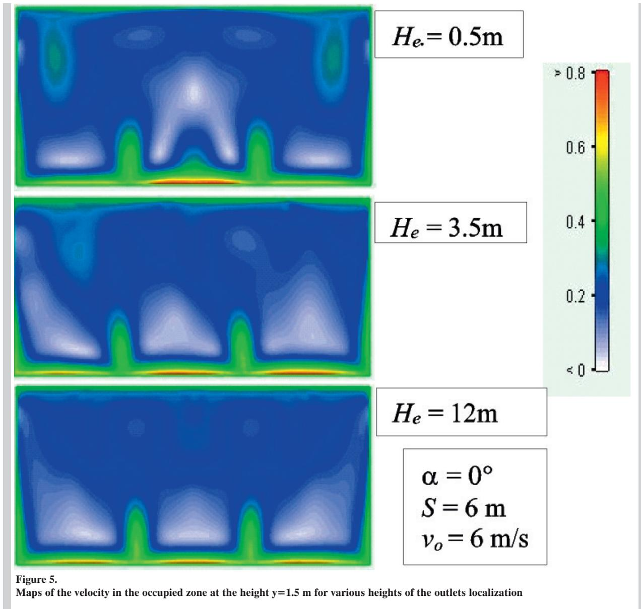
Figure 5. Maps of the velocity in the occupied zone at the height  $y = 1.5\text{ m}$  for various heights of the outlets localization
