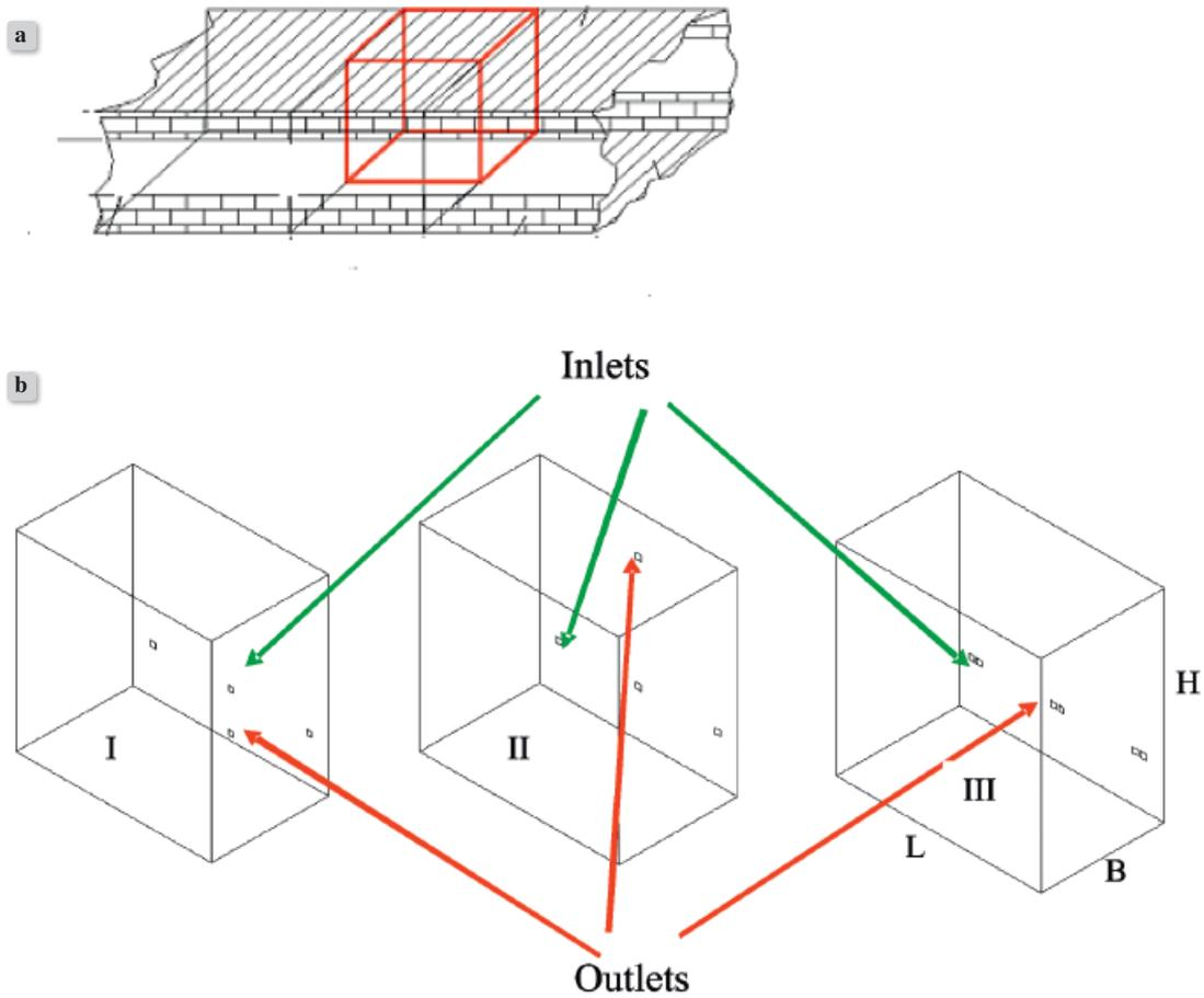
Figure 1. Scheme of the modelled hall a) view of the real object (recurrent module of the entire structure), b) the numerical model for the various localizations of the outlets
