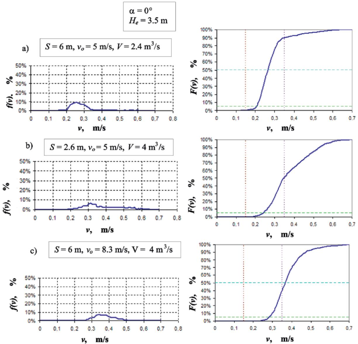
Figure 12. Comparison of the profiles of frequency function and cumulative distribution of speed in the occupied zone for  $y=1.5$  m for various distances of inlets maintaining a constant supply air velocity (a, b) or supply air volume rate (b, c)
