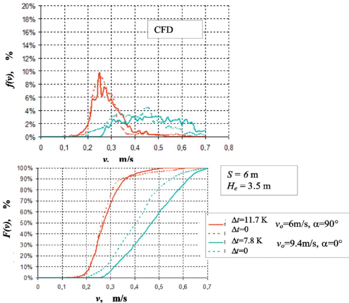
Figure 14. Comparison of the profiles of frequency function and cumulative distribution of speed in the occupied zone for  $y=1.5$  m for isothermal and nonisothermal supply air jet
