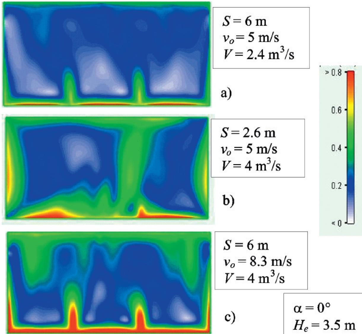
Figure 11. Maps of the velocity in the occupied zone at the height  $y=1.5\text{ m}$  for various distances between the inlets maintaining a constant supply air velocity (a, b) or supply air volume rate (b, c)
