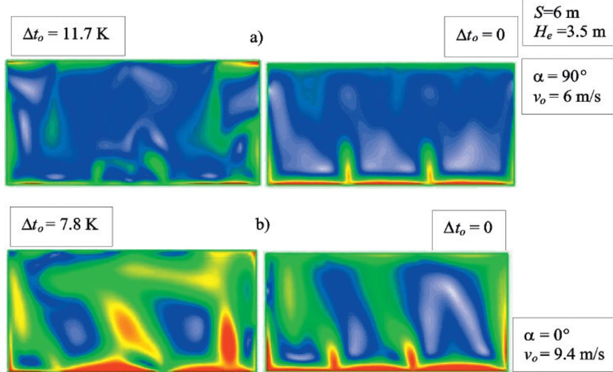
Figure 13. Maps of the velocity in the occupied zone at the height  $y=1.5$  m for isothermal and nonisothermal supply air jet
