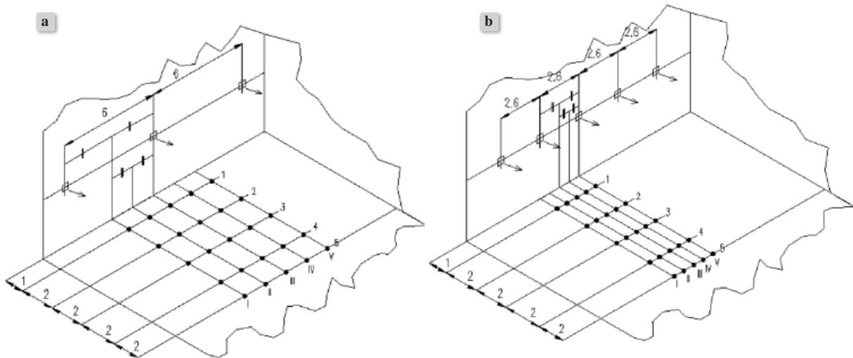
Figure 2. Measurement points in the physical model of the hall in the horizontal plane on the height  $y = 1.5$  m over the floor for two distances between the inlets S a) 6m, b) 2.6m
