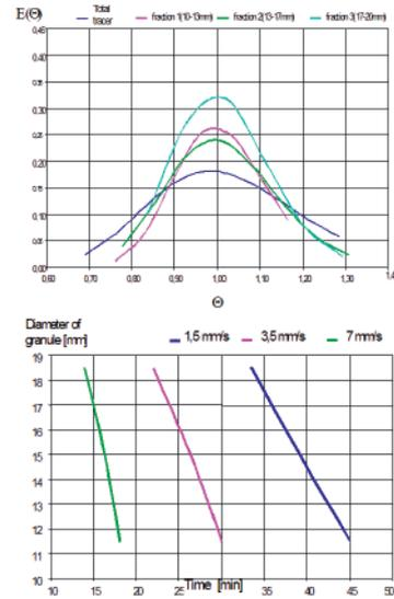
Figure 5. a) Residence time for various fraction of keramsite on the forward moving grate (inclination angle  $13^\circ$ , bars velocity 3,5 mm/s). b) Residence time for various fractions of keramsite for various size of particles and various bars velocity for forward moving grate (inclination angle  $13^\circ$ )
