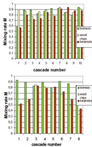
Figure 4. Values of mixing rate of components for: a) forward moving grate, b) reciprocal (reverse) moving grate [9]; where:  $M_b$  - mixing rate of biomass,  $M_{\zeta d}$  - mixing rate of wood chips,  $M_k$  - mixing rate of keramsite
