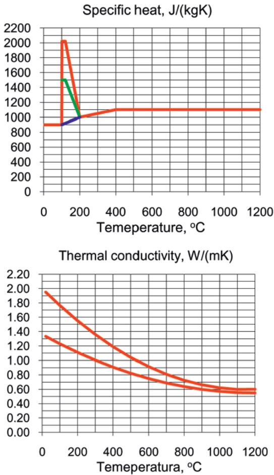
Figure 5. Thermal properties of concrete with siliceous aggregate [3]
