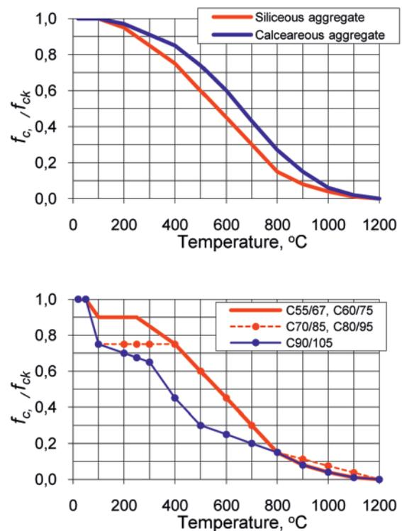
Figure 6. Relative concrete compressive strength decrease in high temperature [3]: a) ordinary strength concrete, b) high strength concrete
