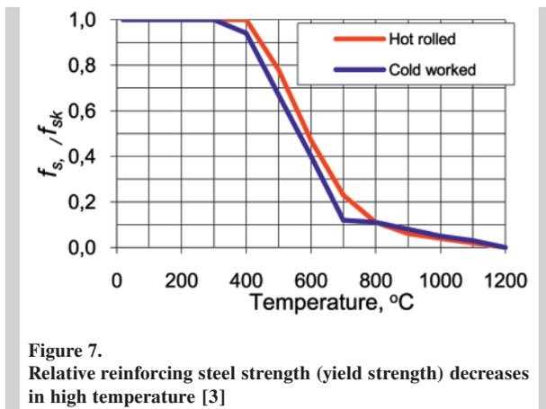
Figure 7. Relative reinforcing steel strength (yield strength) decreases in high temperature [3]
